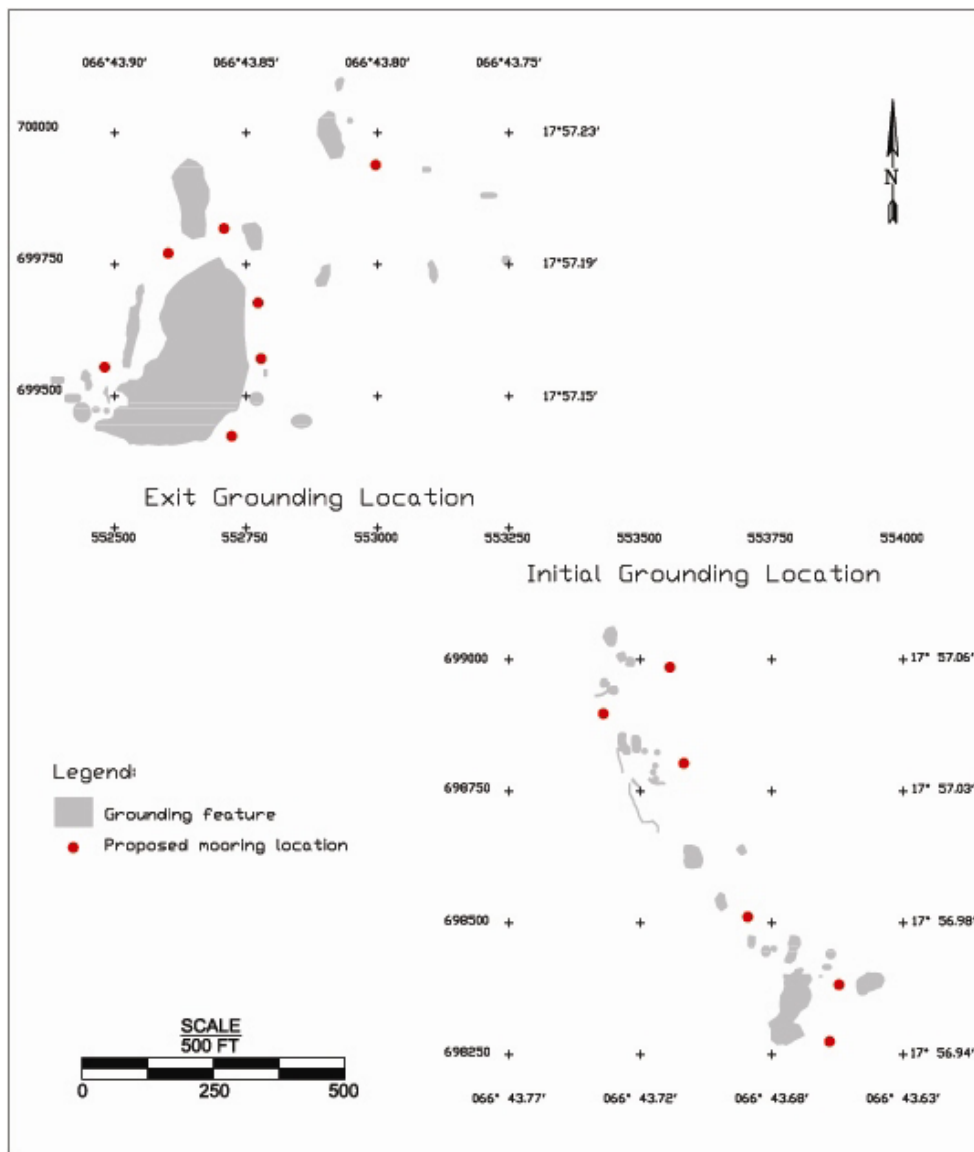
Figure 3. Proposed mooring locations relative to M/T Margara grounding features.
